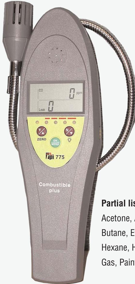
The TPI 775 is a state-of-the-art Carbon Monoxide and Combustible Gas Leak Detector. It is the first of its kind to combine both detection technologies into one easy to use hand-held and affordable instrument.
